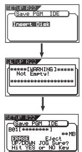
To eject the disc, use the [JOG] dial (or the [CURSOR >] key) to highlight "Eject" then press the [ENTER/YES] key.
