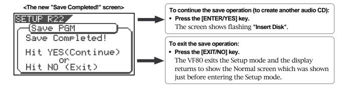
To continue the save operation, carry out either procedures below according to the disc used.
