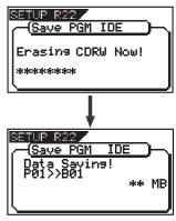
After the erase operation is completed, the save operation immediately starts. When the save operation is completed, "Save Completed!" is shown and the disc is ejected.
