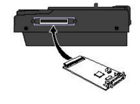
The 8340 card can be retrofit to the VF08's slot on the right side by end-users.
