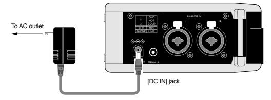
**<Note>:** Do not unplug the AC adaptor while the FR-2LE is accessing a memory card (i.e. during recording, playback, etc.). Turning the power off suddenly may damage recorded data or the memory card.
