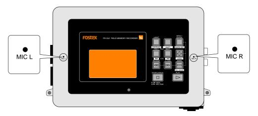
**<Notes>:** Adjust the recording level appropriately so that the corresponding LED level meter on the front panel or on the screen does not exceed "0 dB".
