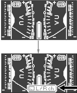
**<Note>**: If you do not press any key for approximately five seconds while the meter mode icon is shown, the icon automatically disappears and the unit exits the meter select mode.
