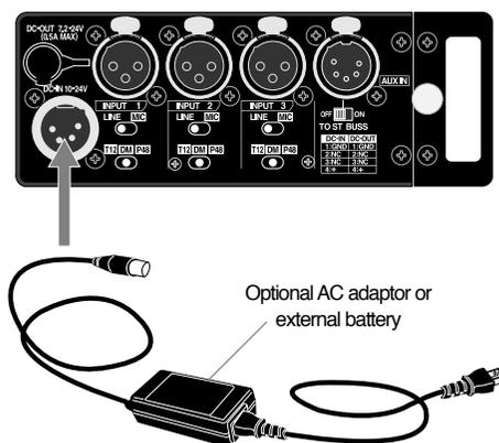
**<Note>**: The rated voltage of the [DC IN] connector is DC 10 V to 24 V. When you connect an external power source to the [DC IN] connector, use the appropriate power source that matches the rated voltage of the [DC IN] connector. For the detail information on the pin assignment of the [DC IN] connector, see page 12 of “Features and controls”.
