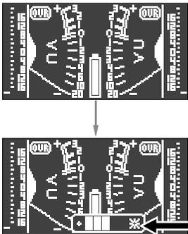
**<Note>**: If you do not press any key for approximately five seconds while the brightness adjustment bar is shown, the bar automatically disappears and the unit exits the display brightness adjustment mode.
