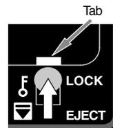
**<Memo>**: To remove the battery box, slide down the [EJECT/LOCK] lever to unlock the battery box. The battery box is slid to the front a few millimeters and you can pull it out by hand.
