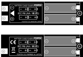
**<Note>**: Always use eight new alkaline or fully charged nickel hydride batteries of the same model and same capacity.
