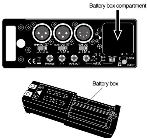
Make sure to set alkaline or nickel hydride batteries to the battery box in correct direction as marked on the box. Set four batteries on each side of the battery box.
