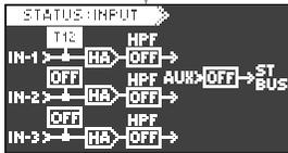
If you set the microphone power supply switch of INPUT 1 to "T12" and set the microphone power supply switches of INPUT 2 and INPUT 3 to "P48", the input status display looks as follows.
