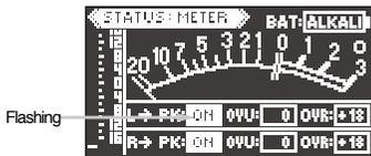
**<Memo>**: By bringing up the meter status display while the unit is receiving a signal, you can edit parameters while checking movement of the VU and peak meters.
