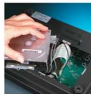
UPGRADABLE HARD DRIVE The removable plate on the underside of a VF80 allows you to change the internal E-IDE hard drive. A larger hard drive means more recording time. Visit www.fostex.co.jp for a list of compatible drives.
