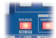
ONE-BUTTON BOUNCING The bounce function allows audio from tracks 1 through 6 to be bounced to tracks 7/8 at the touch of a button.
