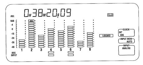
The display example above indicates that the tape position is currently 38 minutes, 20 seconds and 9/100 of a second. The meters show the current level of each playback track. Tracks **4** and **6** are both in
