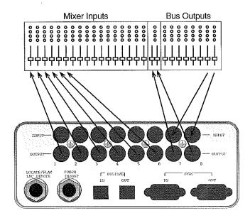
In addition, an external synchronizer connected to the CX-8's [SYNC **OUT**] can output SMPTE or MTC to simultaneously synchronize a MIDI sequencer to tape. This way, you can mix down not only the first 6 tracks
