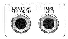
The two footswitch jack functions are designed to be used with any momentary single-pole/single-throw footswitch (either normally open or normally closed). These should be plugged in prior to power-up so that the CX-8 can configure itself for the type of footswitch being used.
