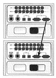
Using the 8-channel proprietary digital bus, you can also bounce tracks between machines in the digital realm. Not only does this result in a perfect copy, but one that is perfectly synchronized with the original. This means you can make perfect safety backups and archives of recordings. One creative way of using a multiple machine system (though it can be done with just one CX-8) is to dedicate two tracks of one machine for stereo
